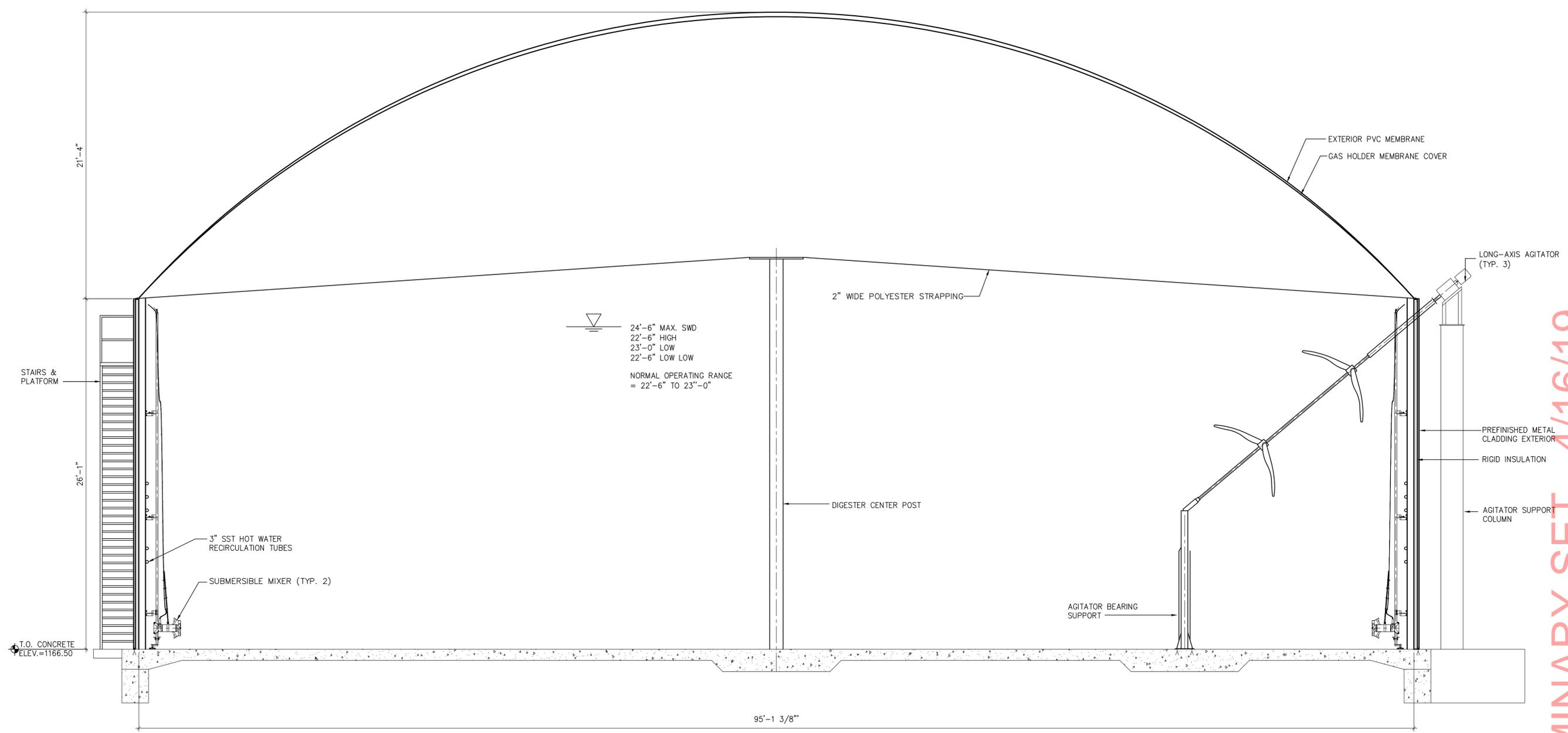
**TYPICAL DIGESTER SECTION** A
